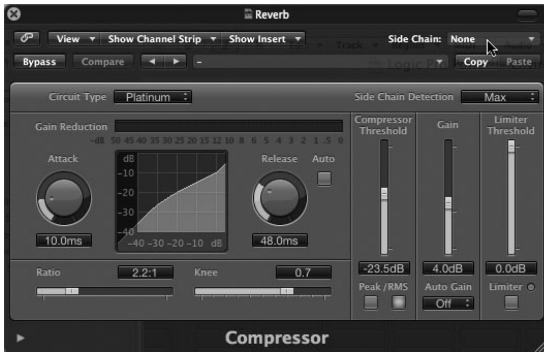
Figure 11.32 The side chain input can be seen on the Compressor effect in Logic as a new pull-down menu on the far right of the control bar.
