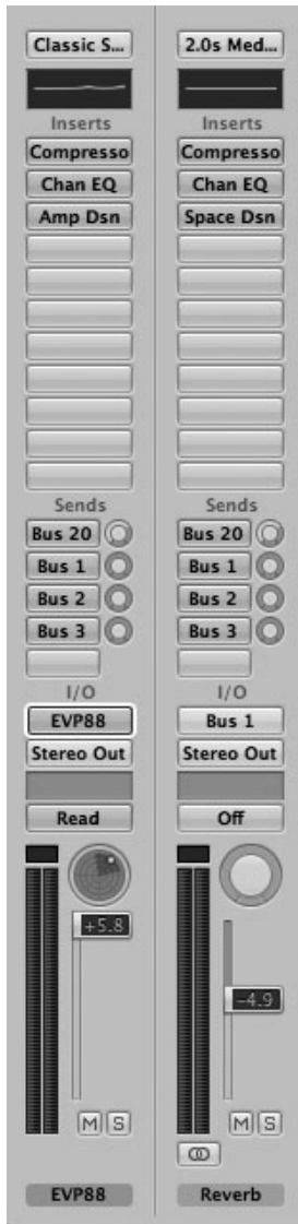
Figure 6.36 The Arrange channel strips of an Audio track. This Software Instrument track is routed through a number of busses, but the Aux channel strip for Bus 1 is displayed to the right. You can select any output on the primary channel strip, and it will display in the second channel strip. As you can see, you'll need to close the Region or Track Parameter box to fit the entire strip on the page on many monitors.
